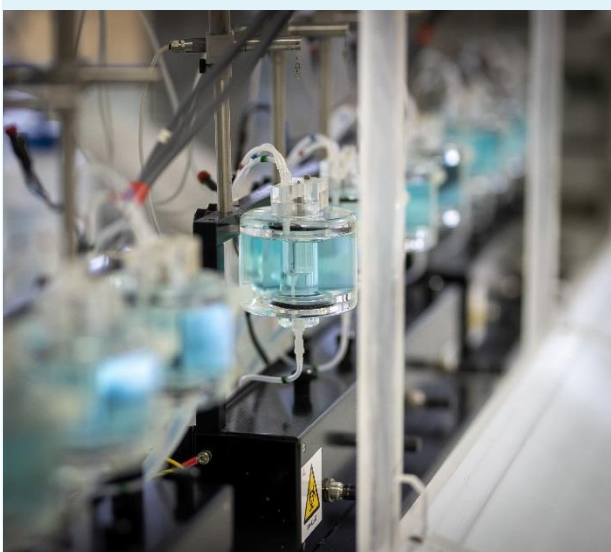
5 mL-organ baths apparatus for ex-vivo functional studies on isolated tissues
