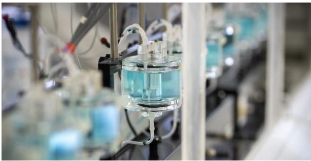
5 mL-organ baths apparatus for ex vivo functional studies on isolated tissues
